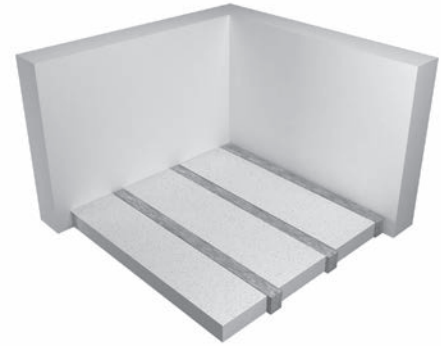
Fit insulation between the joists
